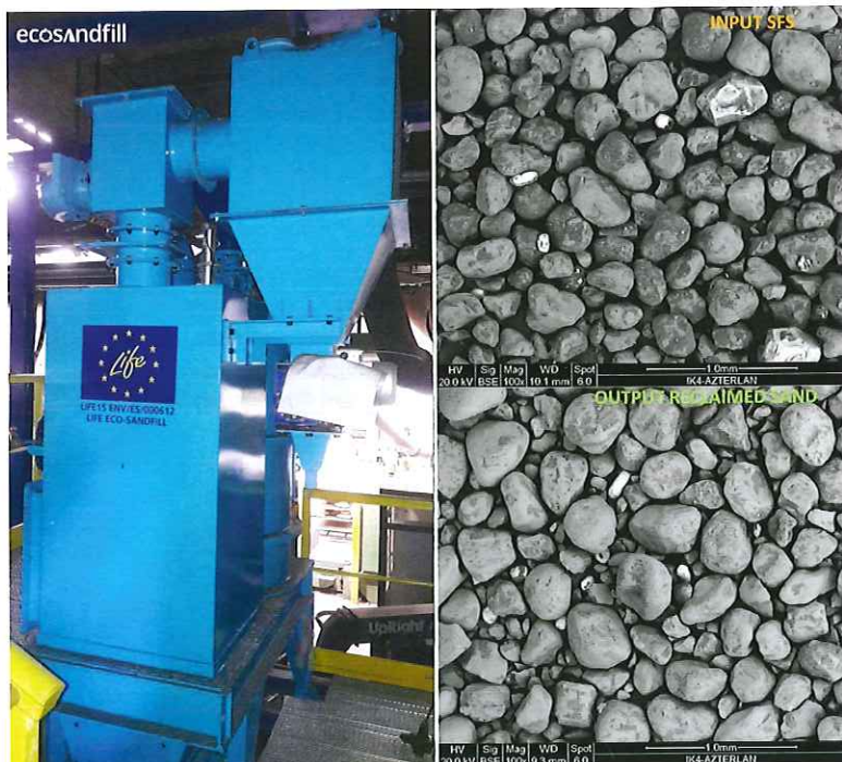
Fig.1 LIFE ECO-SANDFILL reclamation prototype installed at Estanda (left) and compared SEM images (100x magn.) of chemically bonded SFS before (right, top) and after treatment in the system (right, bottom)
